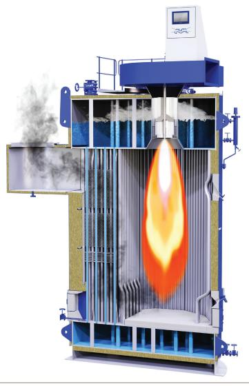
The Aalborg OL is a standard cylindrical two-drum boiler. The furnace, built of membrane walls and containing only little refractory, is shaped to provide optimal combustion conditions. The convection section consists of straight pin tubes with bent pins that provide a high heat transfer coefficient and a low pressure loss. Circulation is ensured by placing downcomers outside the membrane walls.
